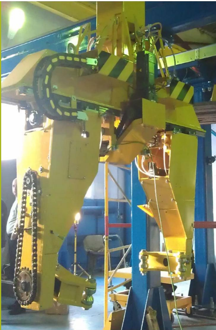
SME Tomsk Electronic Company uses Cartesian manipulators to transport railway wheels
